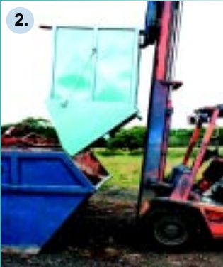
2. Driver then lifts the forks, allowing SUPER-BURRO base to open further. Contents are discharged in a controlled manner.
