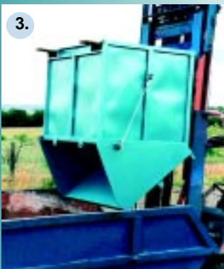
3. Driver can safely lift the SUPER-BURRO to allow full emptying.
